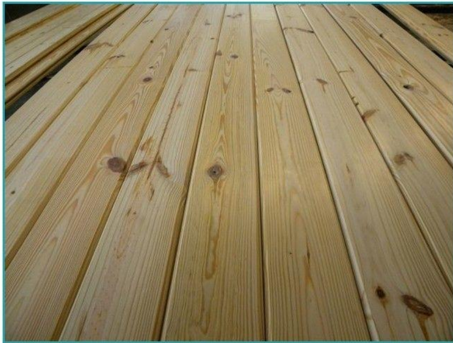
Pine boards of the type used on the roof of the navigating bridge
