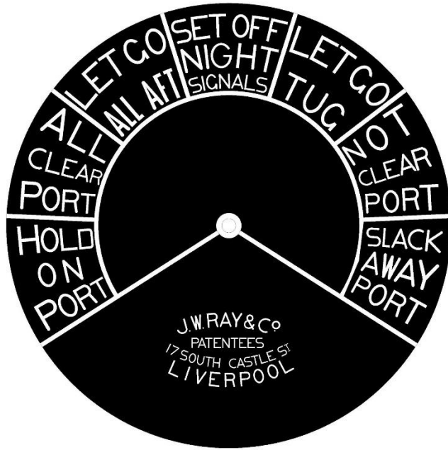
Docking Order Telegraph #2 and #6 Port Dial Face
