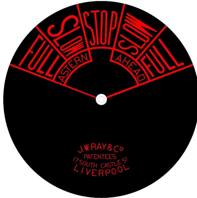
Advisory Engine Order Telegraph #4 Starboard Dial Face
