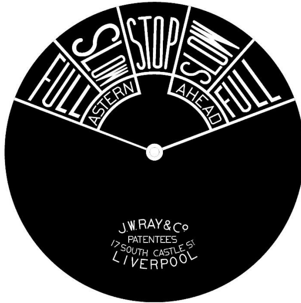
Advisory Engine Order Telegraph #7 Starboard Dial Face
