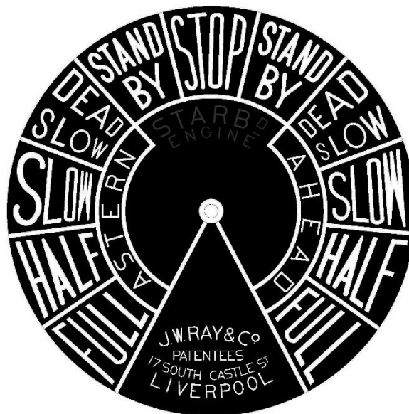
Sauder/Stephenson black and white converted starboard dial face
