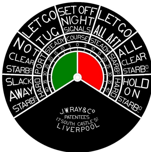
Docking Order Telegraph #2 and #6 Starboard Dial Face
