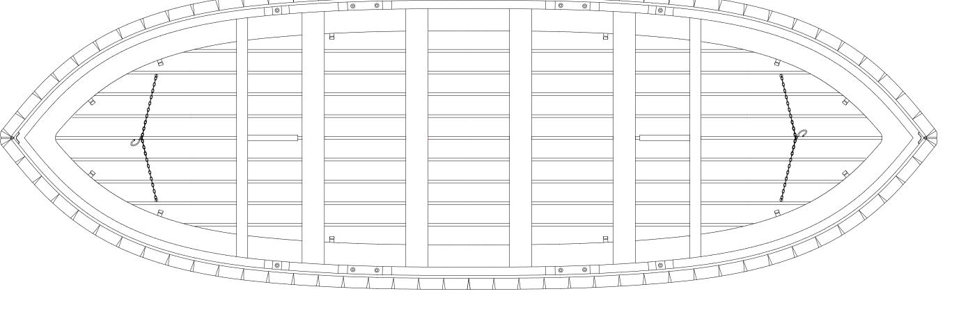
Plan View With Bulwarks Collapsed and Cork Filled Fenders Rigged
